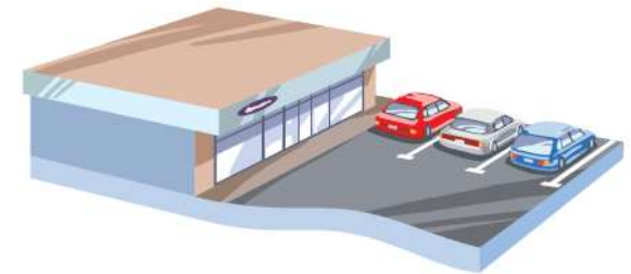
Figure 3: Land required to meet minimum parking requirements is often similar in size to the amount of land occupied by the building.
