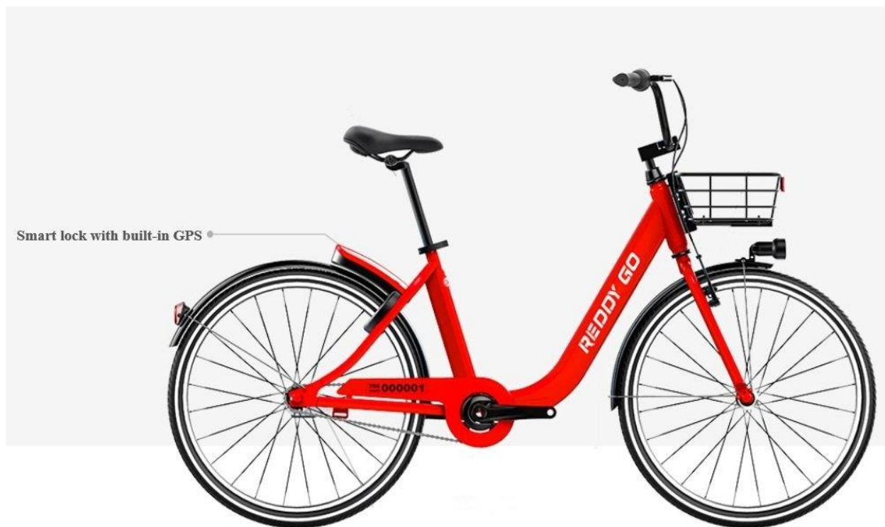
Figure 3. Dockless bike share scheme ‘Reddy Go’ which operates in Sydney and shows the smart lock system on the back on the bicycle.
